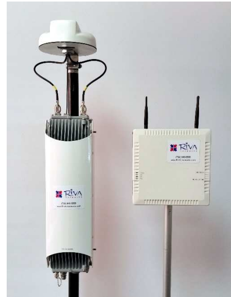
nanoLTE outdoor and indoor radio nodes
